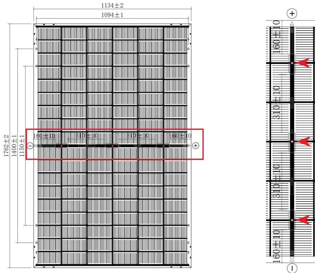
Figure 4: Arrangement of connection boxes using the example of ZEUS 1.0
