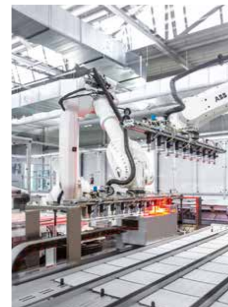
Kamerasystem zum Vermessen der Strings Camera system for measuring selection of strings
